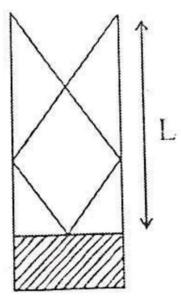
The diagram above show a stationery wave of wavelength 40 cm in a closed tube. The length I is the resonating air column is
