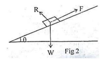
A body of mass 6kg rests on an inclined plane. The normal reaction R and the limiting frictional force is F as shown in the diagram (Fig. 2). If F is 30N and  $g=10\text{ms}^{-2}$ , then the angle of inclination  $\Theta$  is
