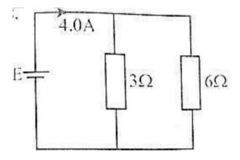
Calculate the e.m.f of the cell in the above circuit if its internal resistance is negligible.
