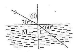
The refractive index of the medium M in the diagram above is
