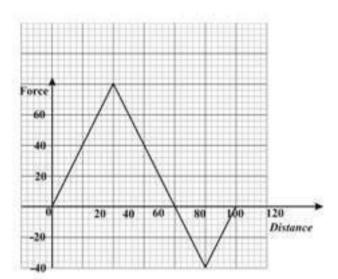
From the diagram above, calculate the work done when the particle moves from x = 0m to x = 80m.
