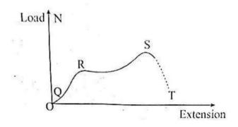
From the diagram above, the point that represent the elastic limit is
