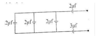
Calculate the effective capacitance of the circuit above
