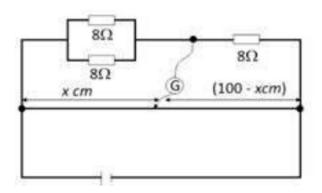
The diagram above shows a balanced metre bridge the value of x is
